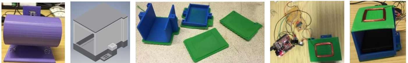
Left: Initial Concept, Middle Left: CAD hardware, Middle Right: 3D printed parts, Right: Completed parts and electronic components
