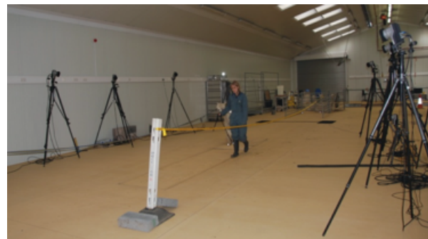
Figure 2 Data collection set-up showing 10 camera optical motion capture system, animal on lead rope and handler in the gait laboratory.
