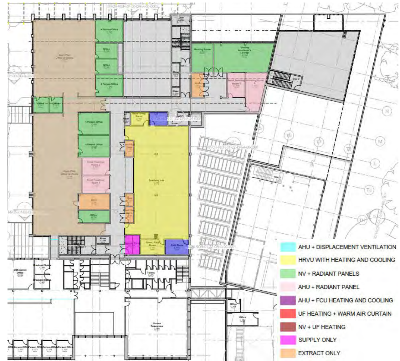
Figure 14: Typical HVAC Strategy - Second Floor
